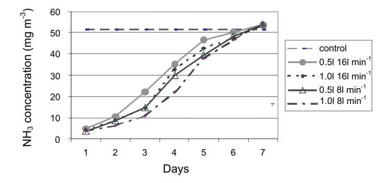
Fig. 3. NH<sub>3</sub> concentrations for the airflow rate 8 and 16 l min<sup>-1</sup> after application of: 0.5 and 1 l of filtration filler, respectively.
