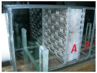
**Fig. 1.** Filtration layer during the experiment – blancking of filler visible.
